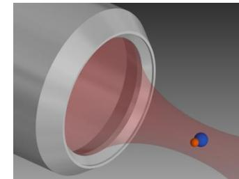
Single fully quantum-state controlled molecule in an optical tweezer
