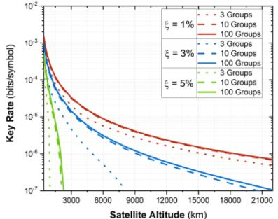
1 GHz,  $V_A = 1$ ,  $\beta = 0.95$ , a = 0.75 m, pointing error 1 µrad, divergence angle 10 µrad, 3 dB fibre coupling loss
