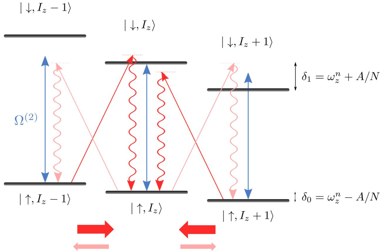
The anharmonic ladder of states leads to a single  $I_z$  determined by two-photon detuning.
