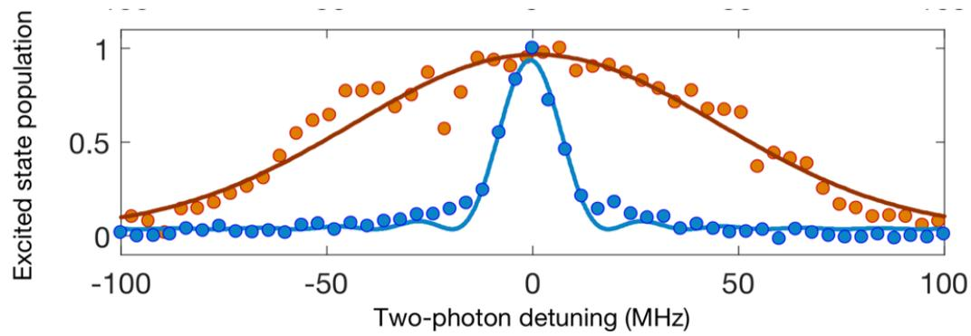
Measured ESR linewidth is  $\sim 15$  MHz  $\rightarrow 400$   $\mu$ K
