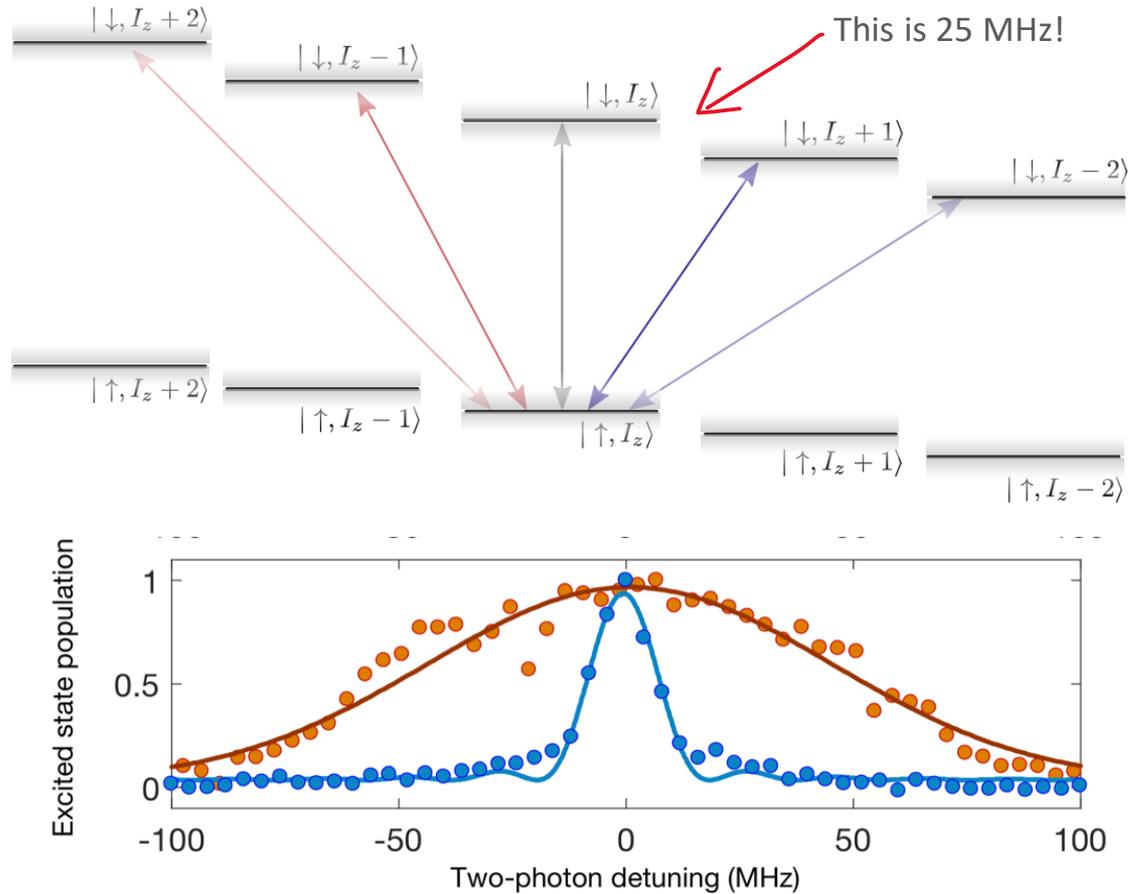
Measured ESR linewidth is  $\sim 15$  MHz  $\rightarrow 400$   $\mu$ K
