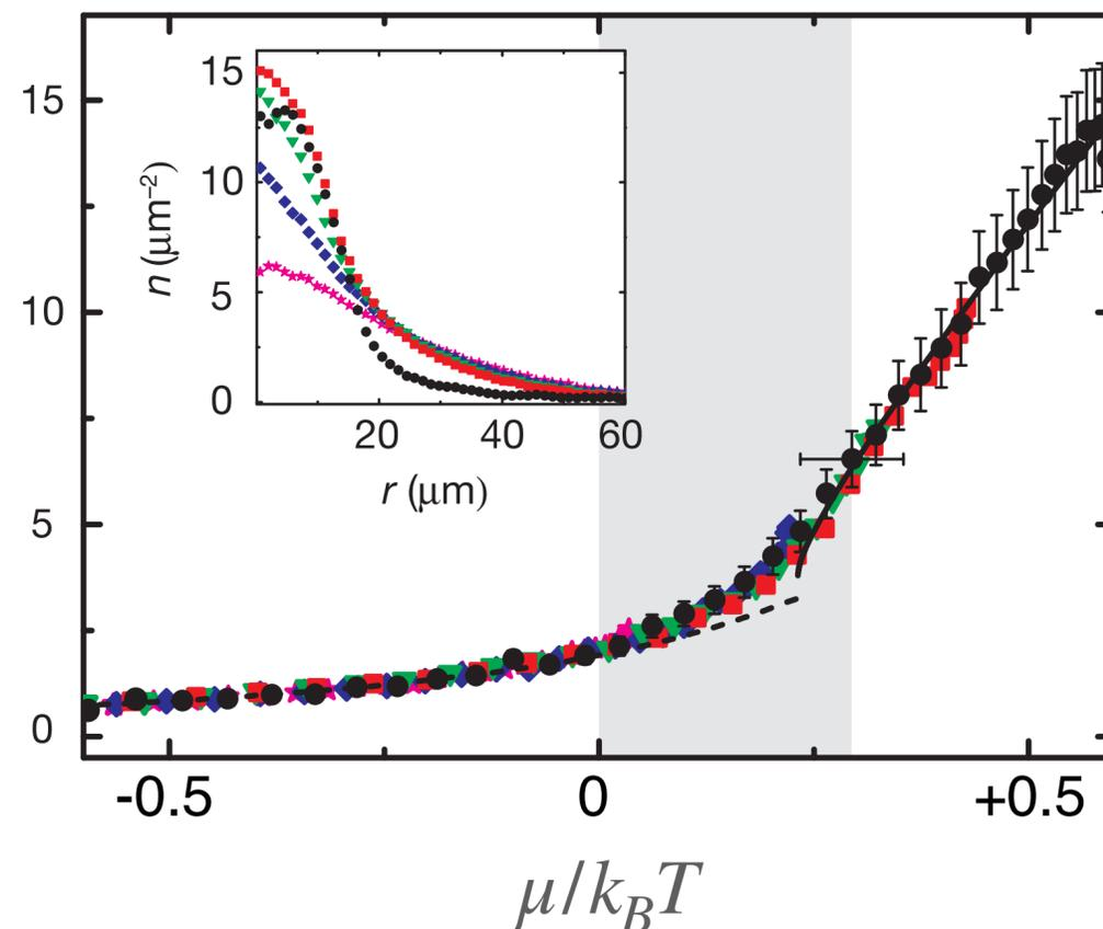
All density profiles obtained for various atom numbers and various temperatures collapse on the same universal curve (for a given interaction strength, here  $\tilde{g} = 0.26$ )
